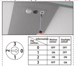
Adjust the dip switch to the module by screwdriver.
